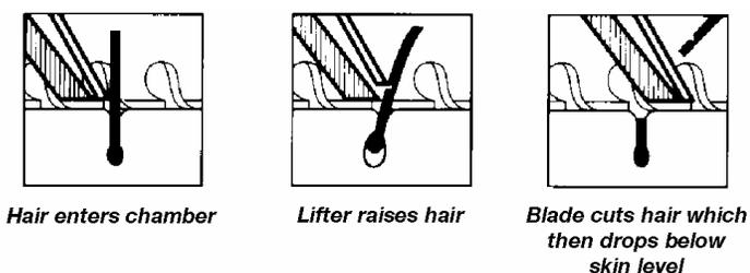
Figure 1. The "Lift-and-Cut" System
